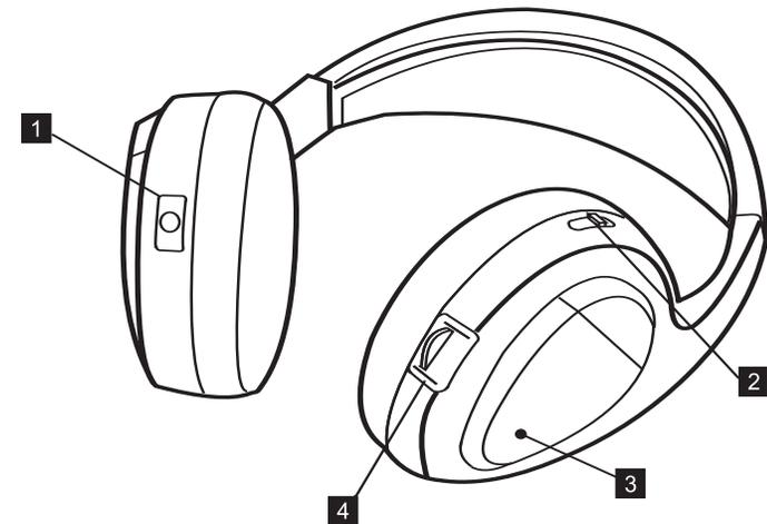
1. **POWER OFF-ON** – Manually turns the headphones on or off. POWER LED will illuminate while the headphones are on.
