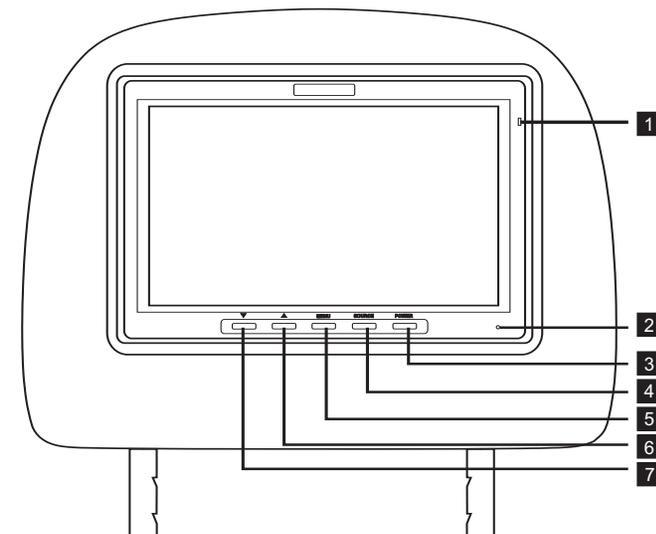
1. **IR Sensor** – Allows the remote to navigate the OSD (On Screen Display) on this unit and to control other functions and accessories.
