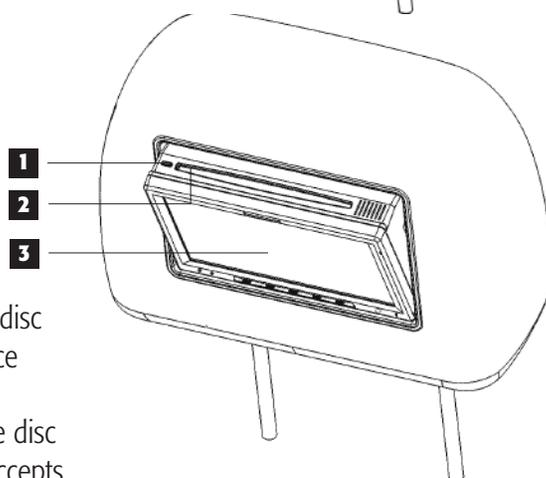
To load a disc, insert the the disc vertically with the label surface facing the rear of the vehicle. Gently lower the disc into the disc slot, until the loader motor accepts the disc and lowers it into the DVD player. Once the disc has been loaded, press on the monitor frame to conceal the DVD loading slot.
