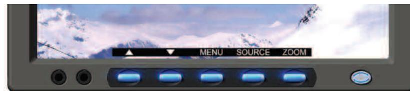
▲ **(UP)** – Increases volume output of wired headphone jack. When in MENU mode also increases the value of the desired function.
