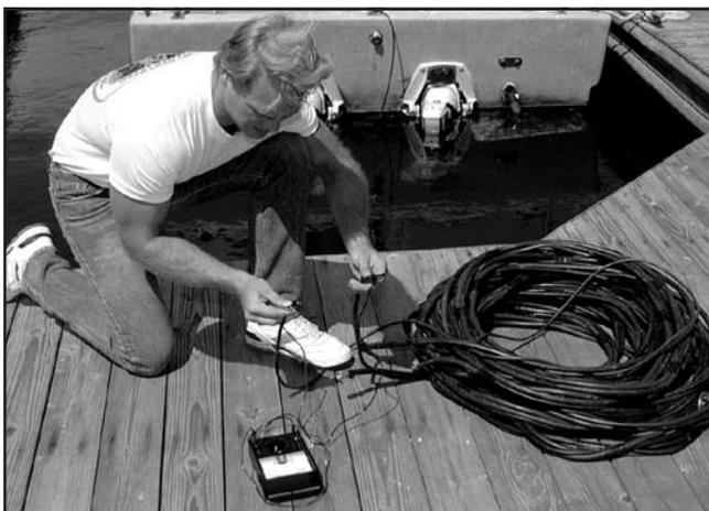
Fig. 8 Preliminary testing of the umbilical with a volt-ohm meter to check for continuity.
