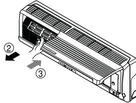
**4** Reinsert air filters and close front panel.
