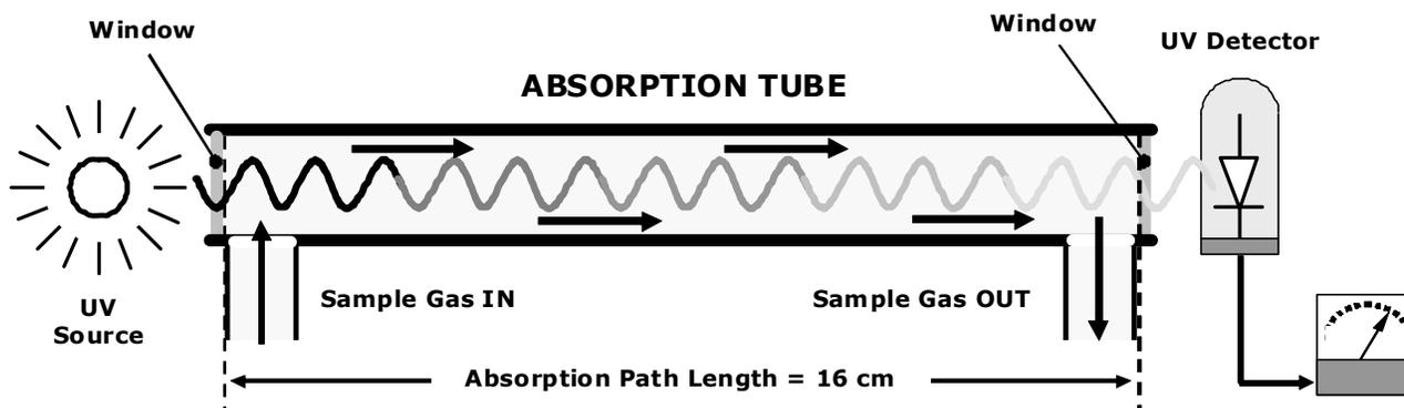
Figure 10-1 O<sub>3</sub> Absorption Path
