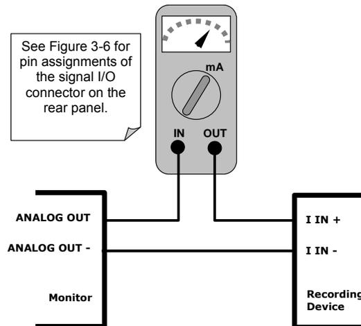
**Figure 8-1 Setup for Measuring Current Output Signal Level**
