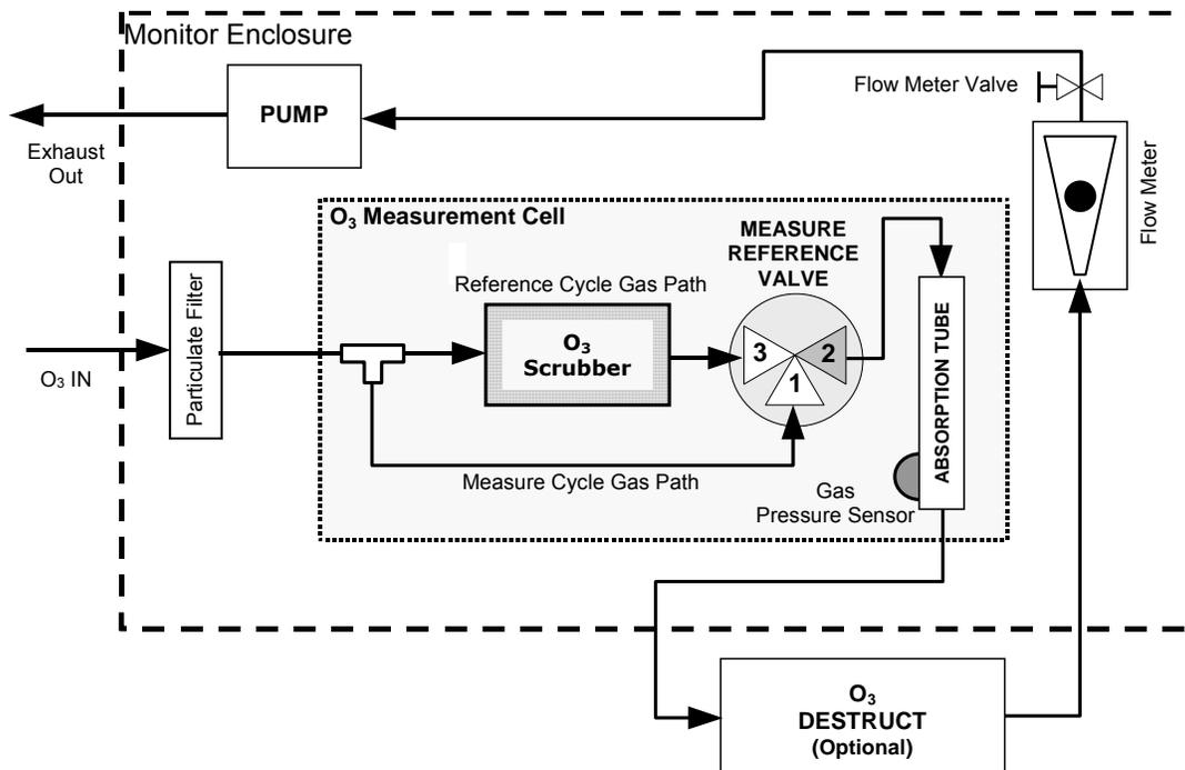
Figure 10-3 460L Internal Pneumatic Diagram – Basic Configuration
