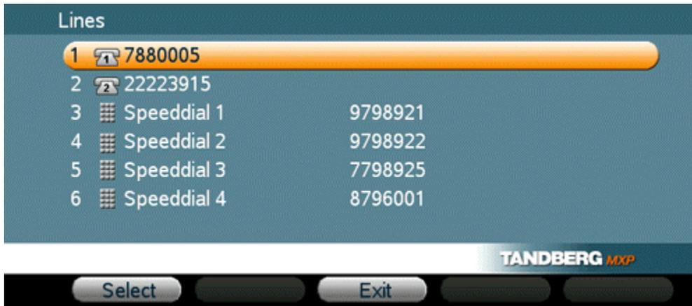
The extension numbers assigned to your unit are shown in the 'Lines' menu. To dial from one of your multiple lines, scroll to the desired line, press the "Select" softkey (or OK), and dial the number you want to reach.
