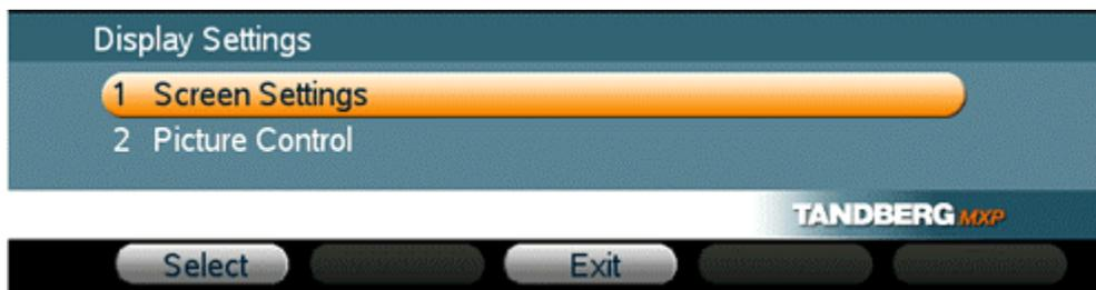
The Display settings menu enables you to configure picture layouts, screen formats, focus, whitebalance and brightness. There are two submenus:
