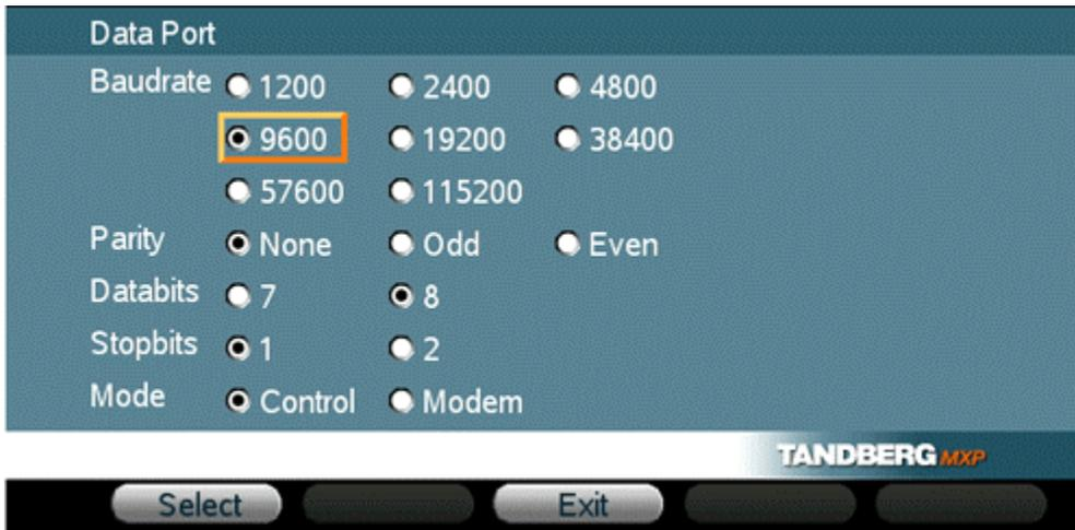
Note that when connecting to a PC the connecting cable must be a straight through RS232 cable.
