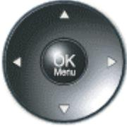
When the menu is hidden, the arrow keys will work on the camera. Hide the menu with the Cancel (X) key and adjust the camera with the arrow keys.
