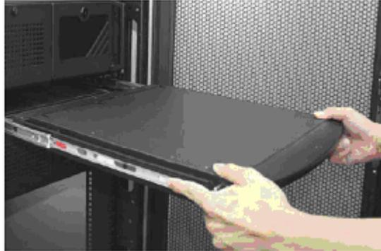
3. Keep pushing the white-arrow buttons until the LCD KVM Console is placed into the rack.
