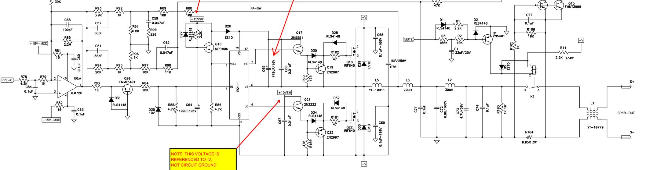
NOTE: THIS VOLTAGE IS REFERENCED TO -V, NOT CIRCUIT GROUND
