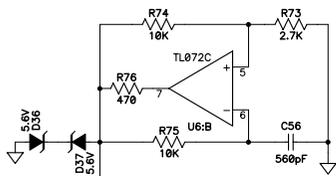
NOTE: THIS VOLTAGE IS REFERENCED TO -V, NOT CIRCUIT GROUND
