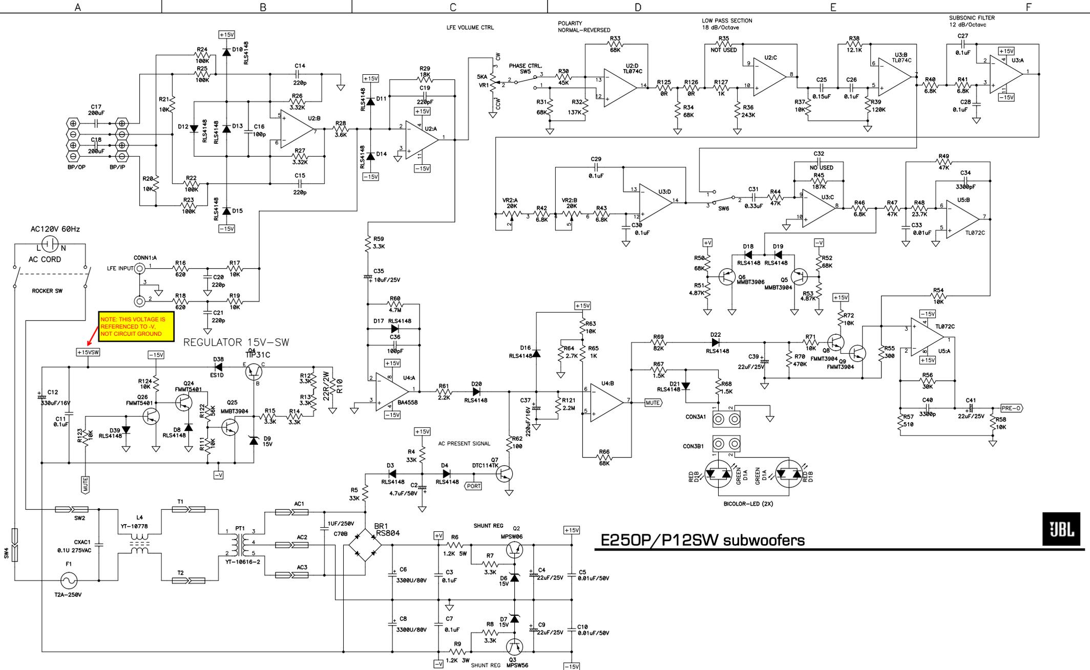
NOTE: THIS VOLTAGE IS REFERENCED TO -V, NOT CIRCUIT GROUND
