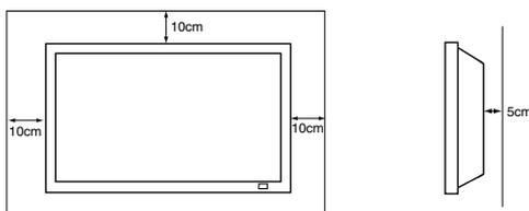
The rear finned section around the cabinet functions as a heat sink, removing heat away from the monitor. The external surface of the cabinet (finned area) must not be covered or the airflow restricted in anyway by enclosing the LCD monitor.
