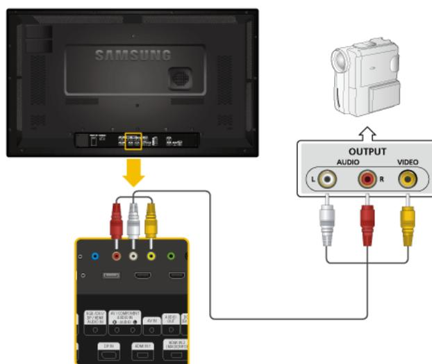
1. Locate the AV output jacks on the camcorder. They are usually found on the side or back of the camcorder. Connect a video cable between the VIDEO OUTPUT jack on the camcorder and the *[AV IN]* on the LCD Display .
