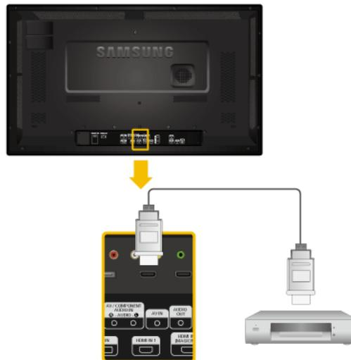
1. Connect an HDMI cable to [HDMI IN 2 (MAGICINFO)] or [HDMI IN 1] on the product and the HDMI output port on a digital device.
