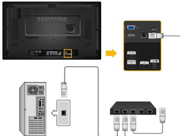
Connect the LAN cable between the [LAN] port on the product and the [LAN] port on your PC.
