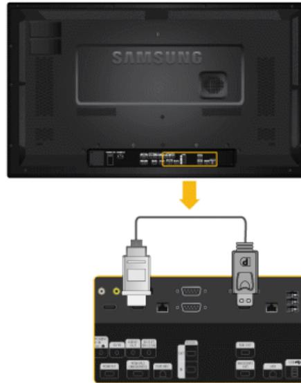
Connect the [MAGICINFO OUT] terminal and the [HDMI IN 2 (MAGICINFO)] terminal on the product using the DP to HDMI cable.
