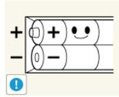
▶ When replacing the battery, insert it with the right polarity (+, -).
