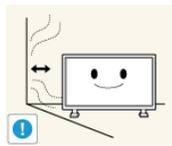
▶ Install your product in a well ventilated location. Ensure that there is a clearance of more than 4 inches (10 cm) from the wall.
