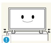
▶ When installing the product in a cabinet or rack, make sure that the front end of the bottom of the product does not project out.
