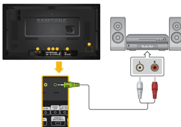
1. Connect a set of audio cables between the AUX L, R jacks on the AUDIO SYSTEM and [AUDIO OUT] on LCD Display.
