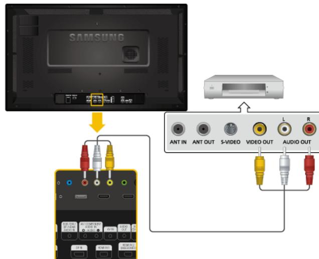
1. Connect an audio cable to *[AV/COMPONENT AUDIO IN (R-AUDIO-L)]* on the product and the audio port on an external device such as a VCR or DVD player.
