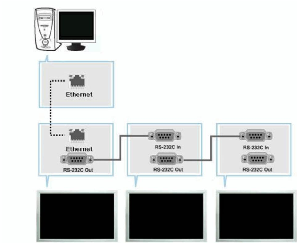
Unlike the previous method which used the serial data communication specifications RS-232C, an Ethernet function has been added. Connect the first display device and the PC by entering the IP address. To connect to another display device, use an RS-232C serial cable. Refer to the figure above.
