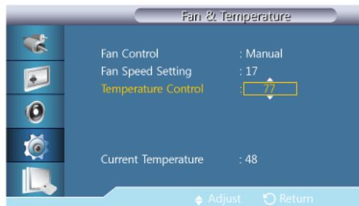
Detects the product's internal temperature and specifies the desired temperature.
