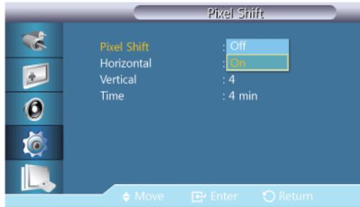
To prevent after-images on the screen, you can use this function to have pixels move on the LCD in the horizontal or vertical direction.
