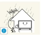
▶ Bend the outdoor antenna cable downwards at the location where it goes in so that rainwater does not flow in.
