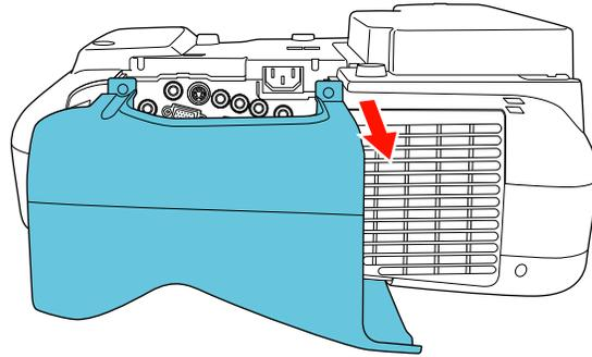
To attach the cable cover, slide it into position, then tighten the screws.
