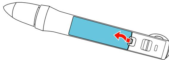
2. Insert the battery with the + and – ends facing as shown.
