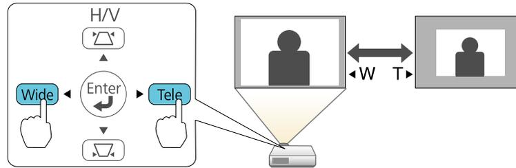
**Note:** If the projector is installed out of reach, you can also adjust the image size using the Zoom setting in the projector menus.
