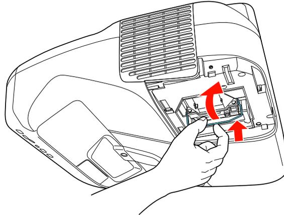
8. Tighten the screws to secure the lamp.
