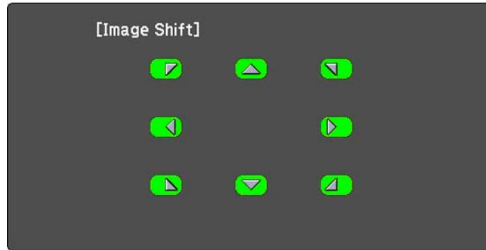
3. Use the arrow buttons on the projector or remote control to adjust the image position.
