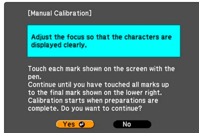
4. Adjust the focus if necessary, by opening the cover on the side of the projector and sliding the focus lever.
