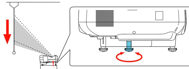
4. If the image is tilted, rotate the rear feet to adjust their height.
