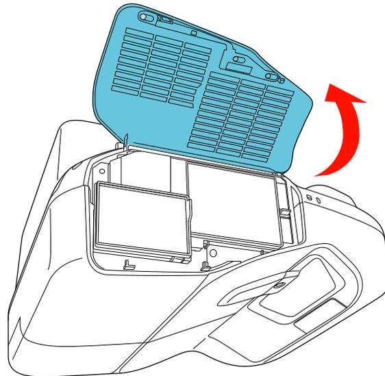
3. Pull the air filter out of the projector.
