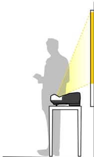
Wherever you set up the projector, make sure to position it squarely in front of the screen, not at an angle.
