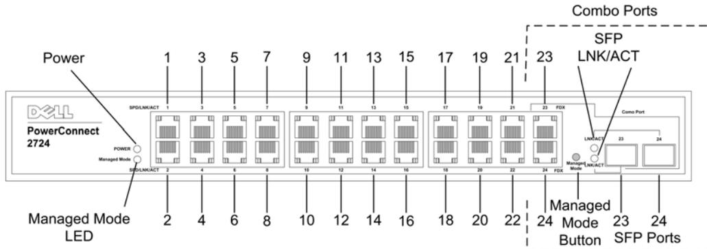
On the front panel there are 24 ports which are numbered 1 to 24, top down and left to right. On each port there are LEDs to indicate the port status. There are two SFP (Small Form-Factor Pluggable) ports, designated as ports 23 and 24, for fiber connection. The two combo ports are logical ports with two physical connections:
