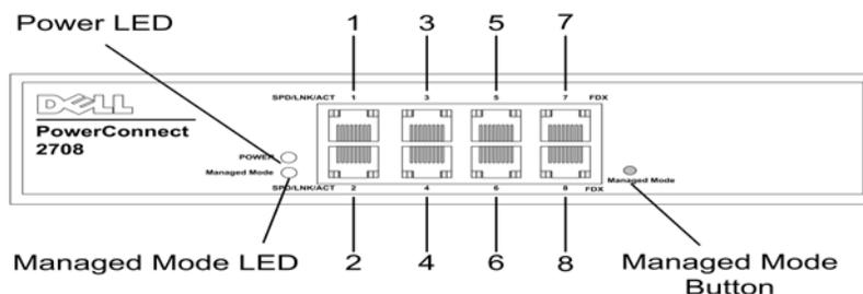
On the front panel there are eight ports which are numbered 1 to 8, top down and left to right. On each port there are LEDs (Light Emitting Diode) to indicate the port status.
