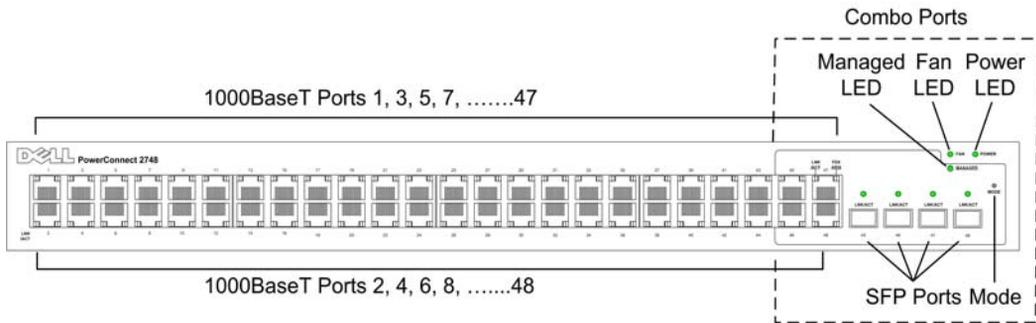
On the front panel, there are 48 ports, which are numbered 1 to 48, top down and left to right. On each port, there are LEDs to indicate the port status. There are four SFP (Small Form-Factor Pluggable) ports, designated as ports 45, 46, 47 and 48, for fiber connection. The four combo ports are logical ports with two physical connections:
