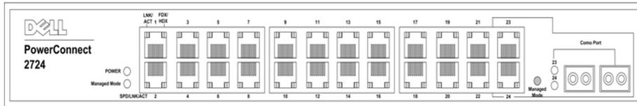
The PowerConnect 2724 switch supports 24 GbE copper ports and has two SFP combo ports (1000BASE-SX or 1000BASE-LX).
