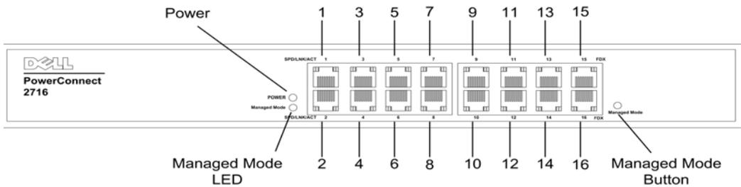
On the front panel, there are 16 ports, which are numbered 1 to 16, top down and left to right. On each port there are LEDs to indicate the port status.
