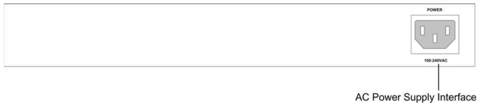
**Figure 2-5. PowerConnect 2724 Front Panel**
