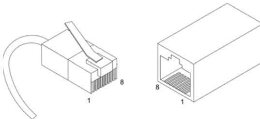
The RJ-45 pin number allocation for the 10/100/1000BASE-T ports is listed in the following table.
