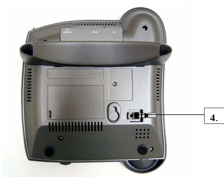
Figure 3. Back Side Panel of the IP Phone
