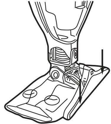
Lift the vacuum nozzle. It should lock into position.
