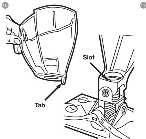
Return the filter to the filter protector and return to the dust canister.
