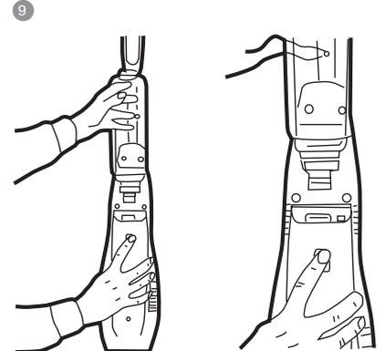
Unscrew the cap from the top of the cleaning solution tank.
