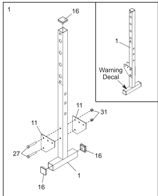
2. Attach the Crossbar (2) to an Upright (1) with two M10 x 68mm Bolts (27), two Joint Plates (11), and two M10 Nylon Locknuts (31). **Do not tighten the Locknuts yet.**
