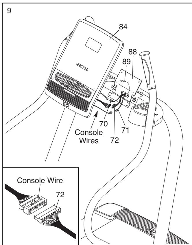
10. Attach the Console (84) to the plate on the Yoke (88) with four #8 x 3/4" Screws (1). **Be careful not to pinch any wires. Start all four Screws before tightening any of them. Do not over-tighten the Screws.**
