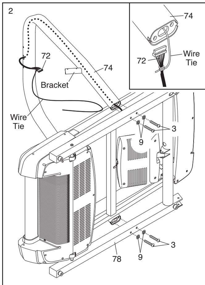
3. With the help of a second person, carefully tip the incline trainer down so that the Base (78) is flat on the floor.
