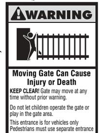
**NOT FOR USE AS PEDESTRIAN PASSAGE!** This operator is intended for vehicular use only. To prevent INJURY to pedestrians, a separate pedestrian access should be supplied, visible from the gate. Locate the pedestrian access where there is not a chance of INJURY at any point during full movement of the gate.
