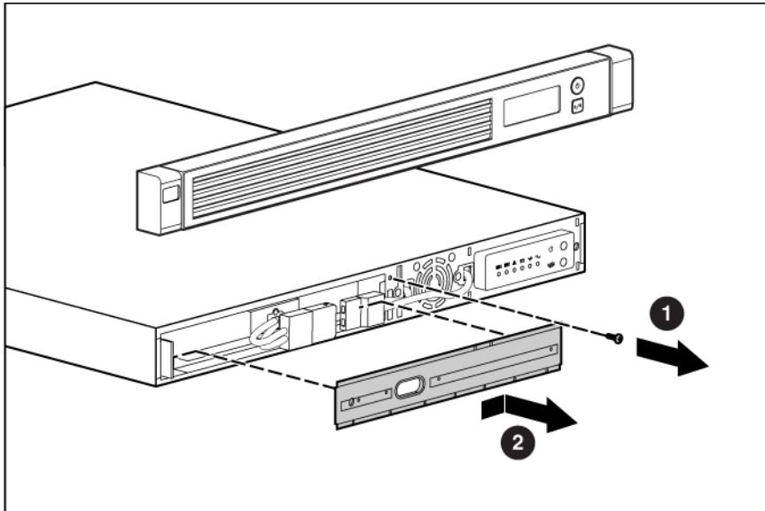
5. Remove the UPS battery modules.
