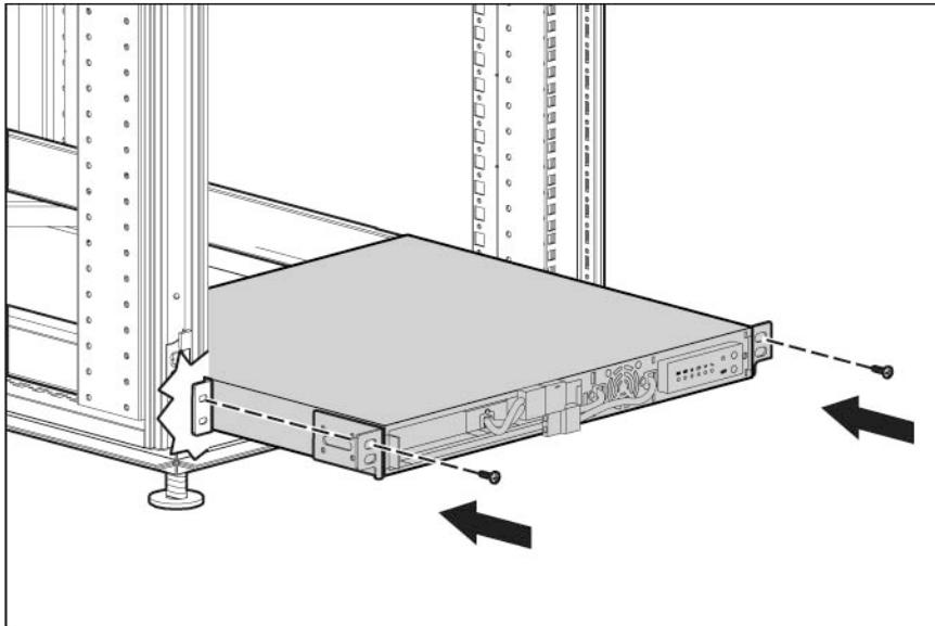
3. (optional) Insert the rear stabilization brackets into the mounting rails and then attach the brackets to the UPS.
