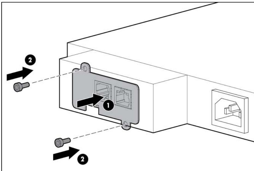
3. Secure the UPS Network Module using the two screws removed in step 1.
