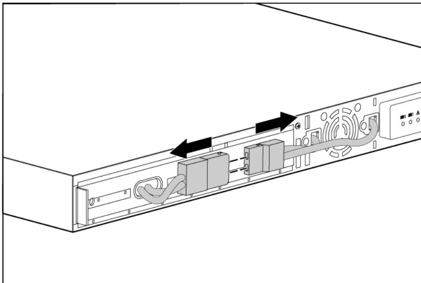
4. Remove the battery bracket.
