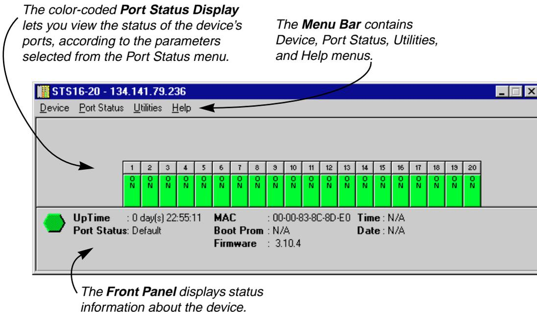
Figure 2-2. The STS16-20 Chassis View Window
