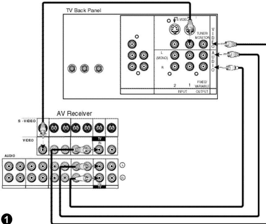
1) Connect a video cable from the Video Monitor Output jack on the back of the AV receiver to the Video Input 1 jack on the television's rear jack panel, using a video plug cable.
