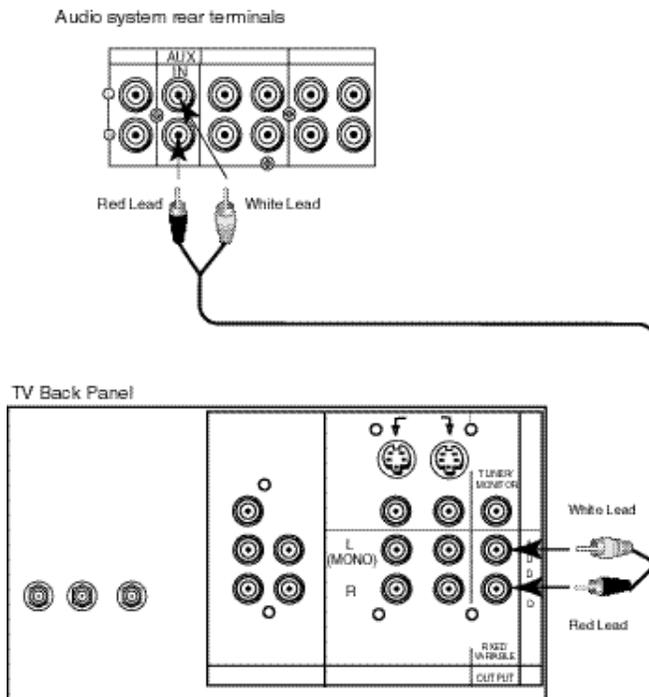
1) Connect the audio cables from the Audio Monitor Output jacks on the television's rear panel to the TV In or Aux In terminals at the back of your audio system. The red cable connects the right Output to the right Input. The white cable connects the left Output to the left Input.
