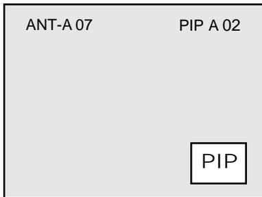
You can also move the PIP window anywhere on the TV screen using the four-way cursor buttons.
