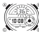
1. In the Timekeeping Mode, hold down (A) until the seconds start to flash, which indicates the setting screen.
