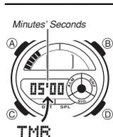
The countdown timer can be set within a range of one minute to 60 minutes. An alarm sounds when the countdown reaches zero. The countdown timer also has an auto-repeat feature and a progress beeper that signals the progress of the countdown.
