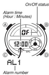
You can set five independent Daily Alarms. When an alarm is turned on, the alarm tone sounds when the alarm time is reached. One of the alarms is a snooze alarm, while the other four are one-time alarms. You can turn on an Hourly Time Signal that causes the watch to beep twice every hour on the hour.
