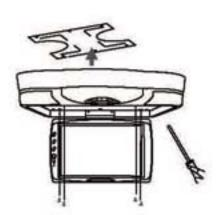
Flip the monitor screen down and tighten the monitor to the support bracket, using the supplied screws.
