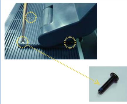
Remove 4 screws and then remove hinge.
