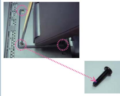
Remove 4 screws and then remove hinge.
