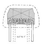
You may adjust the stainless steel by adjusting the tube until the headrest indicator can fit on the back seat. (Maximum adjustment width is 4CM)
