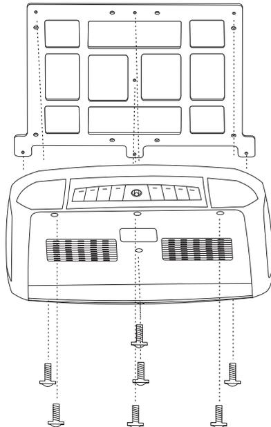
4. Tighten the unit with the supplied screw B.
