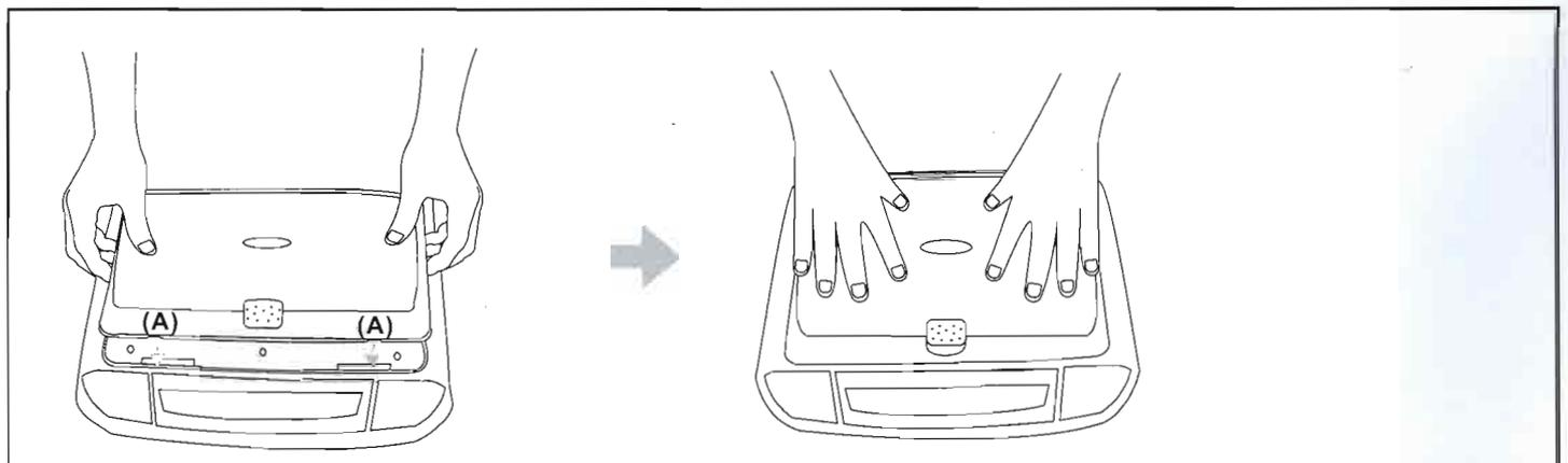
Open the screen and hook the two tabs (A) on the bottom edge of the screen. Snap the opposite side over the hinge.
