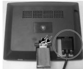
Power Connector in VGA Cable for LM-2110
