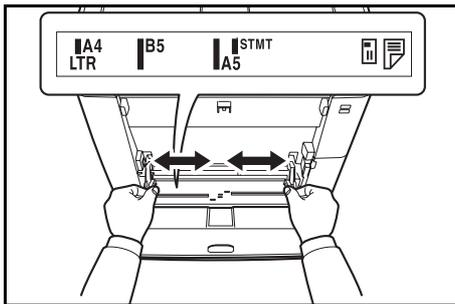
3 Adjust the position of the paper guides on the MP tray. Standard paper sizes are marked on the MP tray or Manual Feed tray. For standard paper sizes, slide the paper guides to the corresponding mark.
