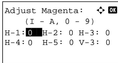
**10** In the color registration correction chart printed in Print Registration Chart above, note the numbers of the sections in the magenta H and V charts where the lines most closely coincide as a single straight line. In the left example, the value would be B.
