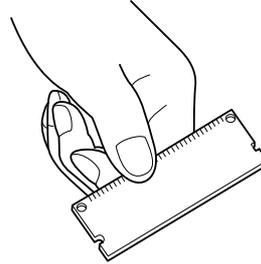
To protect electronic parts, discharge static electricity from your body by touching a water pipe (faucet) or other large metal object before handling the memory module. Or, wear an antistatic wrist strap, if possible, when you install the memory module.
