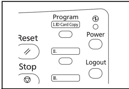
**ID Card Copy** is printed on the **Program 1** key. When the functions are deleted by overwriting **Program 1** key, seal the label supplied with the machine and write the function name in it.
