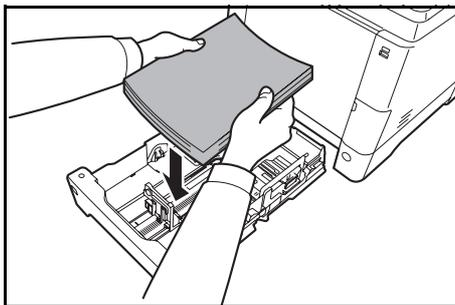
**5** Load the paper in the cassette. Ensure the side to be printed is **facing up** and the paper is not folded, curled, or damaged.
