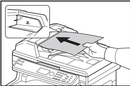
Ensure that loaded originals do not exceed the level indicator. Exceeding the maximum level may cause the originals to jam (see the figure).
