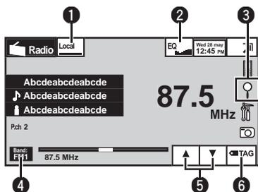
Manual tuning (step by step) using the buttons
