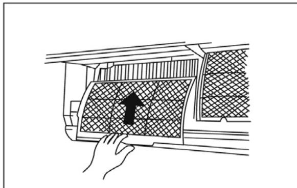
4. Remove the air freshening filter (optional on some models) from its support frame
