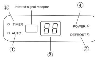
**NOTE:** For cooling only models  $\geq 18000$ Btu/h indicator light ② is for FAN ONLY, not defrost.
