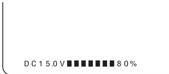
The battery voltage information is displayed all the time when ON has been selected as the BATTERY REMAIN item setting on the OSD screen of the main menu.
