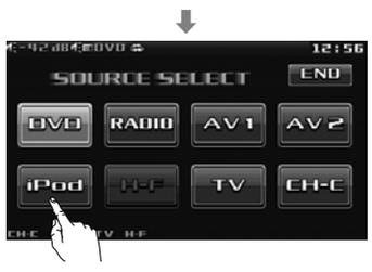
② Touch (iPod) on the Source Selection Screen. (Content varies with connected devices)
