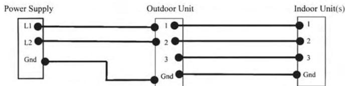
**NOTE:** For Multi-zone systems, there are two sets of identical wiring terminals. Be sure to match each air handler with its corresponding terminal strip connection. Use above diagram for each circuit.
