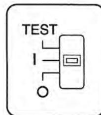
**To STOP:** Turn the Hand Switch Lever to OFF "O" position.
