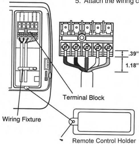
4. Fix the connecting wire between units, with wiring fixture.
