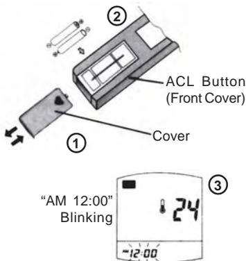
1. To lift the cover press in and up on the lid latch with your thumb nail.
