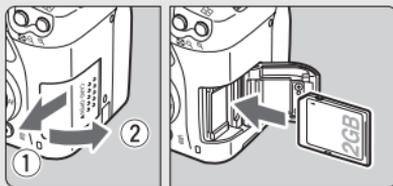
**Open the slot cover and insert a card.** (p.31)
