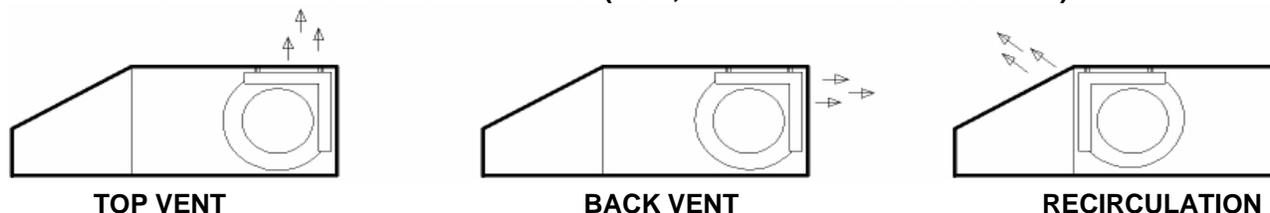
**IMPORTANT NOTE: If hood is to be vented out the Top or Back, the charcoal filters must be removed.**
