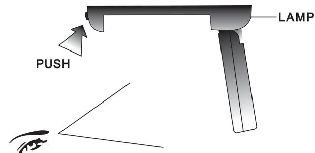
Eject monitor set by pressing PUSH button and then, adjust monitor set for your comfortable watching.
