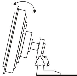
A.When you install the monitor into the seat head cushion make sure that the monitor connecting cable assembly has already been pull through by the supporting pipe.
