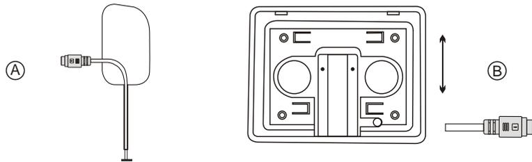
Note: Installing Method of main cable assembly
