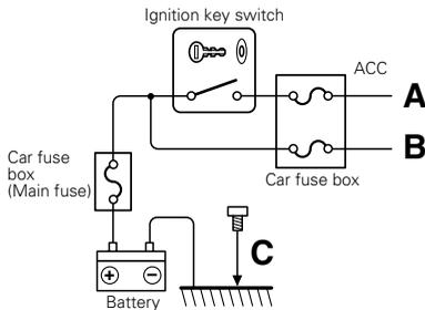
Depending on what antenna you are using, connect either to the control terminal of the motor antenna, or to the power terminal for the booster amplifier of the film-type antenna.
