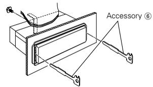
4. Lower the removal tool toward the bottom, and pull out the unit halfway while pressing towards the inside.
