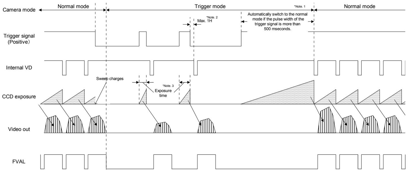
Note 1: The camera does NOT switch to normal mode when the long exposure mode is selected.
