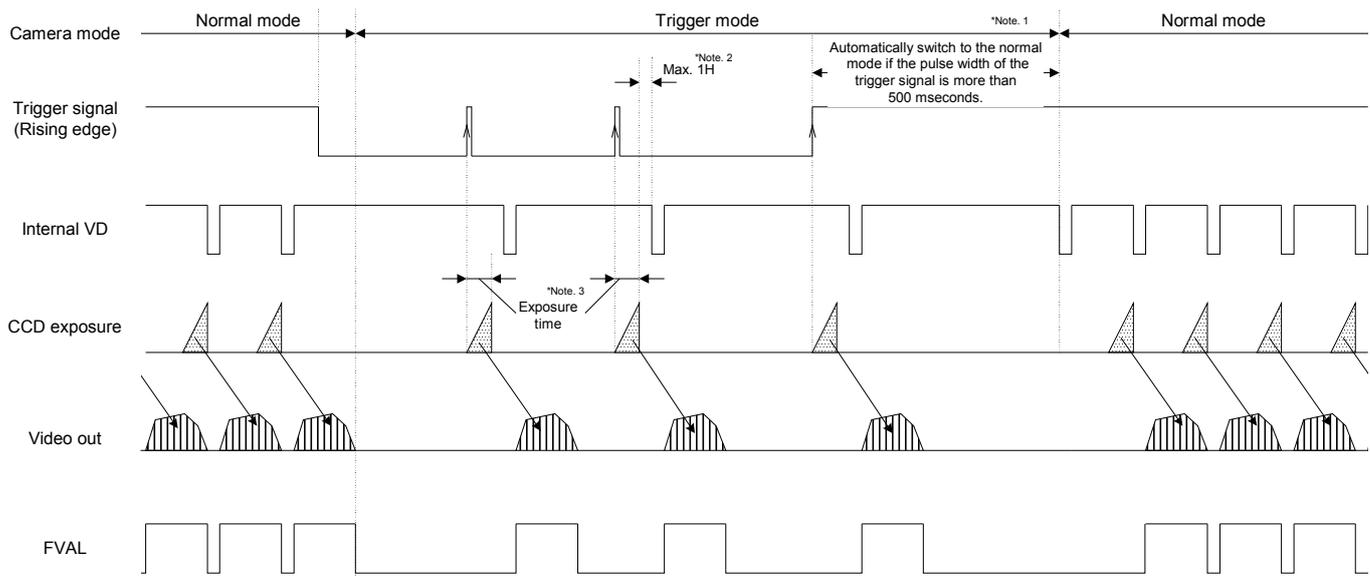
Note 1: The camera does NOT switch to the normal mode when the long exposure mode is selected.
