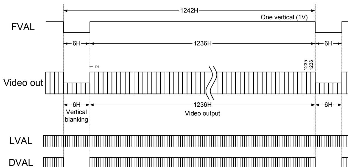
※ By transferring the blanking period pixels at a high rate, the frame rate of the partial full scanning can be increased compared to that of the normal full scanning.
