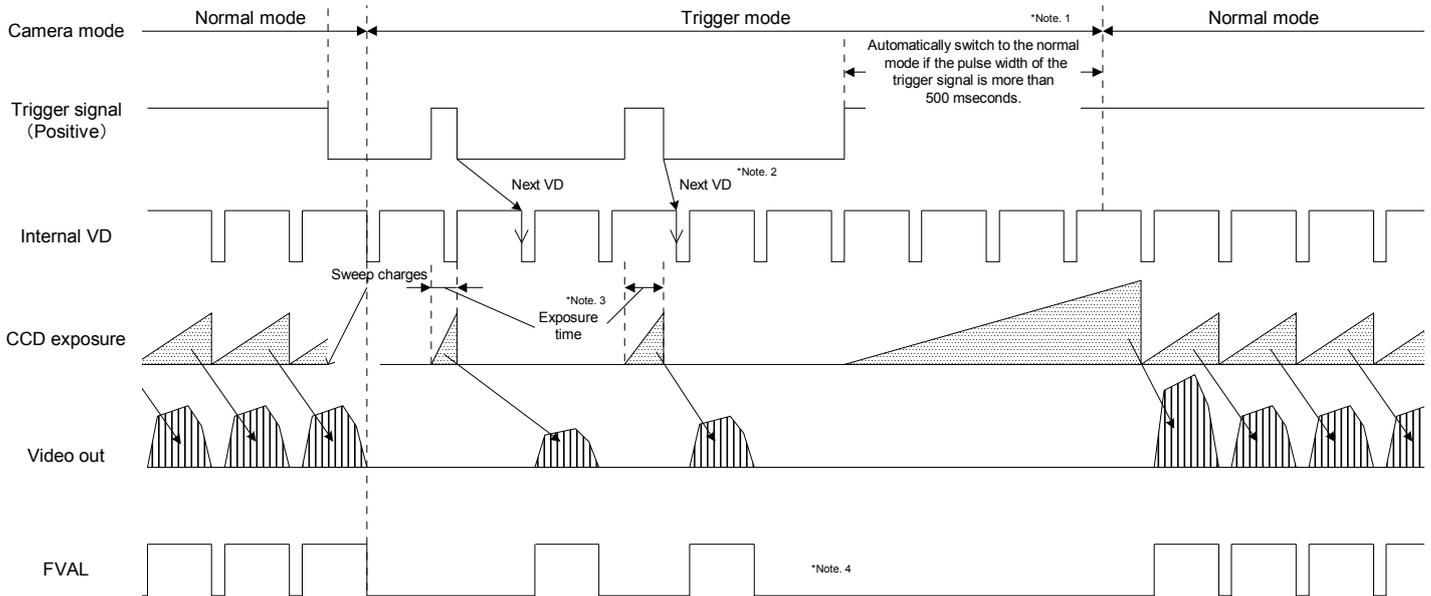
Note 1: The camera does NOT switch to normal mode when the long exposure mode is selected. This timing chart shows with the long exposure mode selected.
