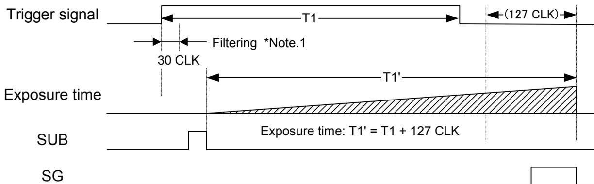
Notes: The trigger signal equal to or shorter than 30 CLK is removed by the filtering system. Input trigger signal has to be more than 31 CLK pulse width. The exposure starts 101 CLK after the rising edge of the trigger signal.
