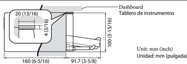
Install the unit at an angle of less than 30°.
