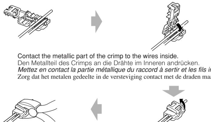
Contact the metallic part of the crimp to the wires inside.
