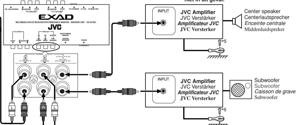
\*5 Firmly attach the ground wire to the metallic body or to the chassis of the car—to the place uncoated with paint (if coated with paint, remove the paint before attaching the wire). Failure to do so may cause damage to the unit.
