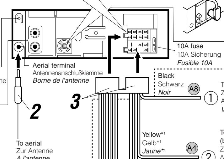
\*1: Before checking the operation of this unit prior to installation, this lead must be connected, otherwise power cannot be turned on.
