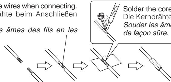
Solder the core wires to connect them securely.
