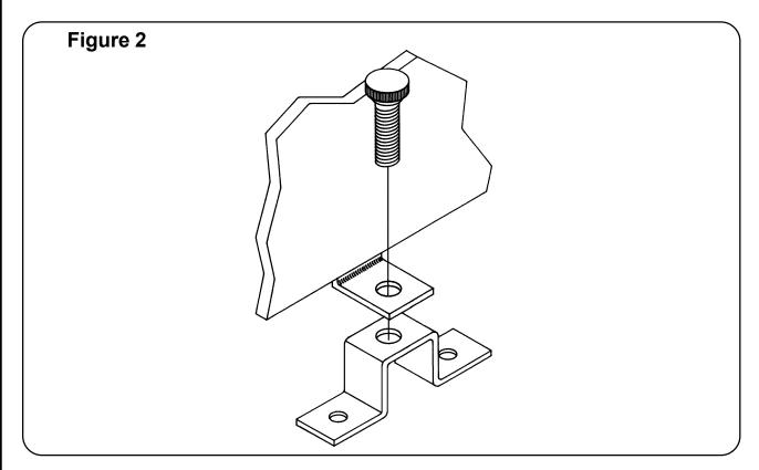
Set the console on the floor of the vehicle and mark where the eight (8) holes of the U-shaped brackets are to be drilled. (Make sure that you have checked under the vehicle and in the vehicle floor (under the carpet) for obstructions)
