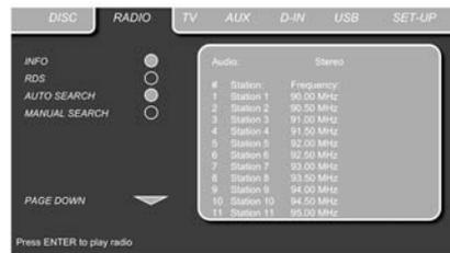
The Radio menu shows the selected Audio mode, the name of a station currently played (as long as RDS is available) and a Station list listing the 30 stations with their preset, station name and frequency.
