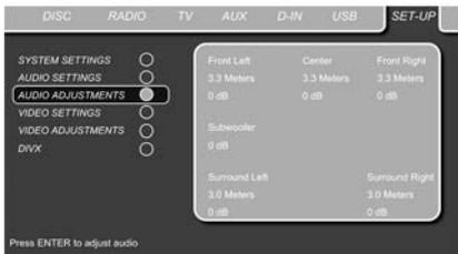
The Audio Adjustment submenu contains the access to the speaker delay and the output level adjustment settings of the CS3/CS5. Follow the explanations in the Upper Menu Line on the bottom of your screen to make adjustments.
