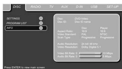
In DVD and MP3 mode, activating the Disc Info (DVD) or ID3 Info (MP3) submenu will show information about the player and the disc currently playing. The first lines will show Disc Type and Disc ID. Below you can compare the Aspect Ratio, Video Standard and Scan Type available on the disc with the actual output of your player or ID3 info for MP3 files.
