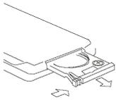
1. Press the catch and at the same time pull out the battery tray.
