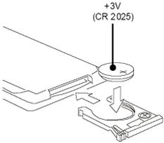
2. Insert the 1 x lithium battery, type CR 2025 3V battery with the stamped (+) mark facing upward. Insert the battery tray into the remote control.
