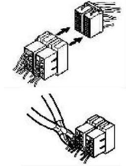
1. If your car is equipped with the ISO connector, then connect the ISO connectors as illustrated.
