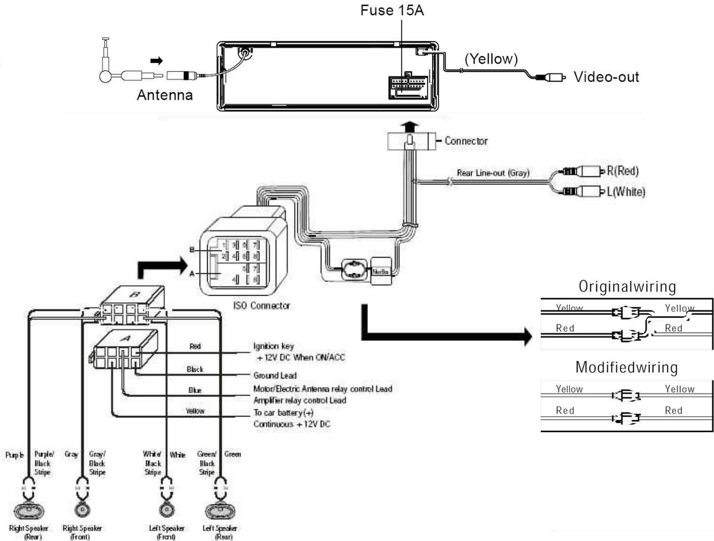
Do not interchange the connection of the wiring!!!
