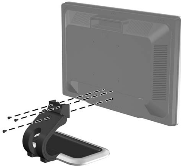
Figure 3-17 Removing the Single-Hinged Pedestal Base
