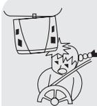
Do not mount the product where it will obstruct the deployment of the airbag or in an area where it would affect the driver's ability to control the vehicle. Also be careful to avoid mounting the product where it can become hazardous during sudden stops or in the event of an accident.
