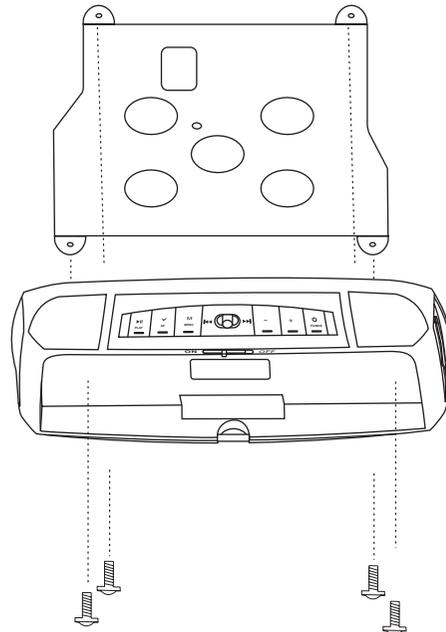
4. Tighten the unit with the supplied screw B.
