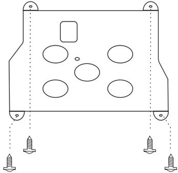
3. Match the position of installation bracket and installation plate with screw A.
