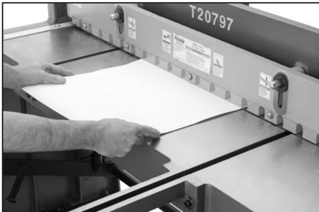
Figure 31. Example of a paper shear test.
