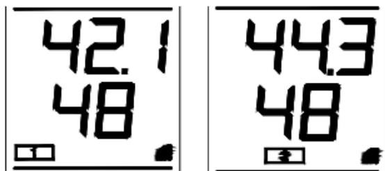
2. To view the Minimum/Maximum temperature: first select from which remote temp/humidity sensor to read data from (indicated by the “boxed” number). Pressing and releasing the “MIN/MAX” button will toggle through the minimum and maximum indoor temperature, and the minimum and maximum outdoor temperature.
