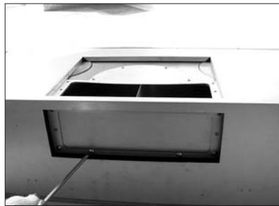
E. Remove the pre-mounted rectangular plate.
