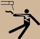
Disconnect electric power to the unit before cleaning the condenser.
