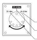
This switch limits the autofocus range to speed up focusing in each
